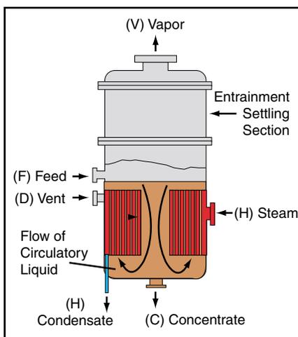
■ Figure 3. In a short-tube vertical evaporator, the process liquid is inside the tubes and the heating medium outside the tubes.
