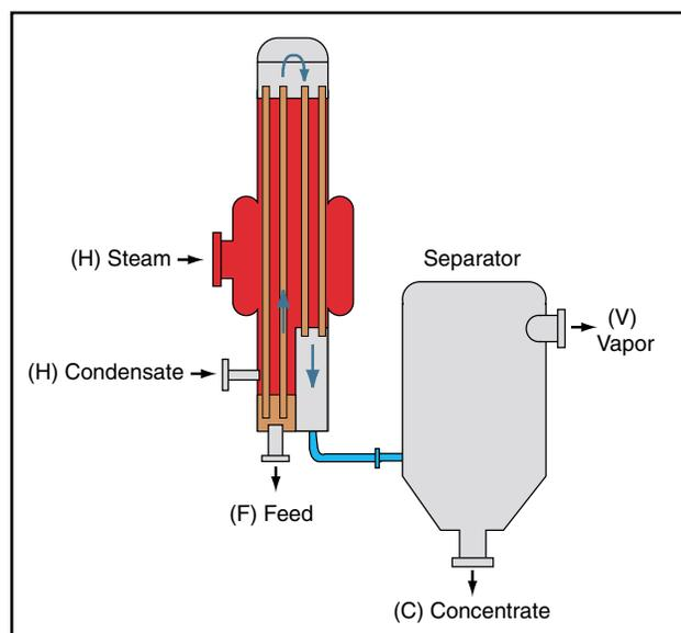
■ Figure 6. A rising/falling-film evaporator combines the advantages of both the rising-film and falling-film designs.
