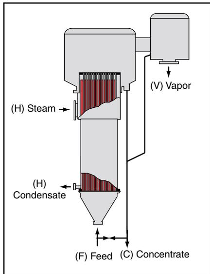
■ Figure 4. Feed flows upward through the tubes and heating medium flows downward on the shellside of a long-tube rising-film vertical evaporator.
