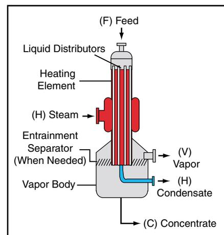
■ Figure 5. The falling-film evaporator is a variation of the long-tube rising-film design, in which the tubular heat exchanger is on top of the liquid/vapor separator.
