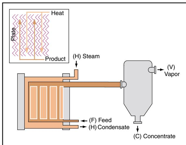
■ Figure 7. A gasketed plate-and-frame evaporator may be operated in a rising-film, falling-film, or rising/falling-film mode.
