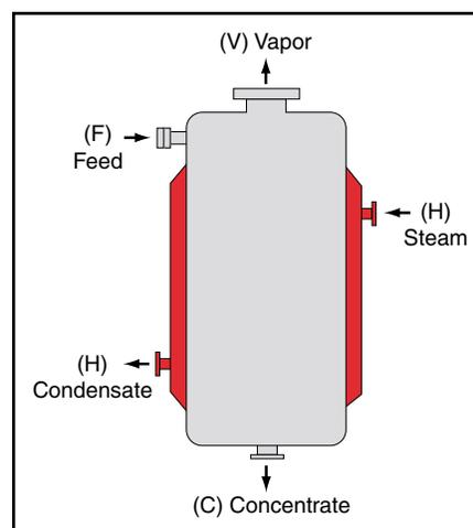
■ Figure 1. A batch evaporator is one of the simplest designs.
